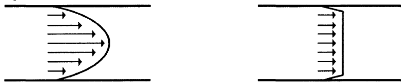
[Figure 7] Illustration of the flow-profiles associated with pressure-driven and electrically driven separation methods. The parabolic profile linked to pressure-based separation methods results from the discontinuous pressure gradient is created by the frictional drag experienced along the capillary edges. 65
