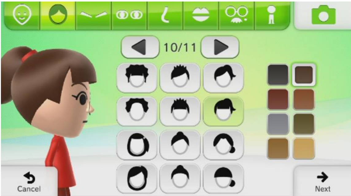
Figure 44. Hairstyle options are represented by buttons with simplistic representations or "glyphs" of each hairstyle. Here, a Mii has been rotated, revealing what the back of the hairstyle shown in the above figure looks like from the side.
