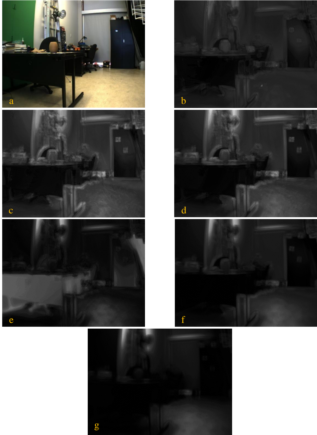
Figure 3.9: A sequence of the AIM saliency maps using a various number of features. a) is the original image, and b-g) are the saliency maps using 7, 25, 69, 163, 251, and 478 features respectively.
