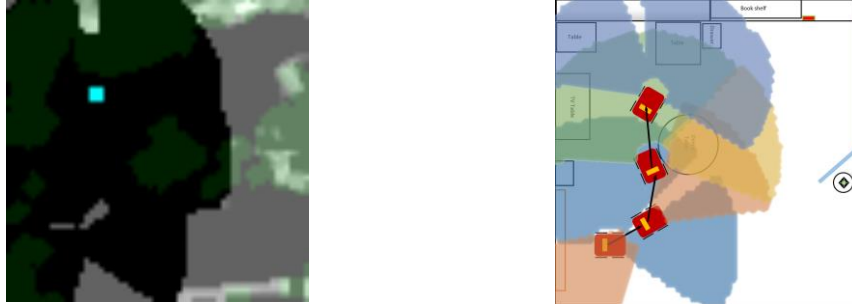
Figure 5.31: The search using the EGS algorithm with the time constraint. From the left to right, a 2D representation of the 3D probability distribution map and the top view of the environment. The robot finishes the search and fails to find the target.
