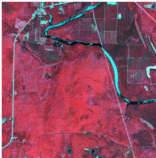
Figure 3.8. False colour composite of Quickbird Image. Quickbird band 2 set to blue, band 3 set to green, band 4 red.
