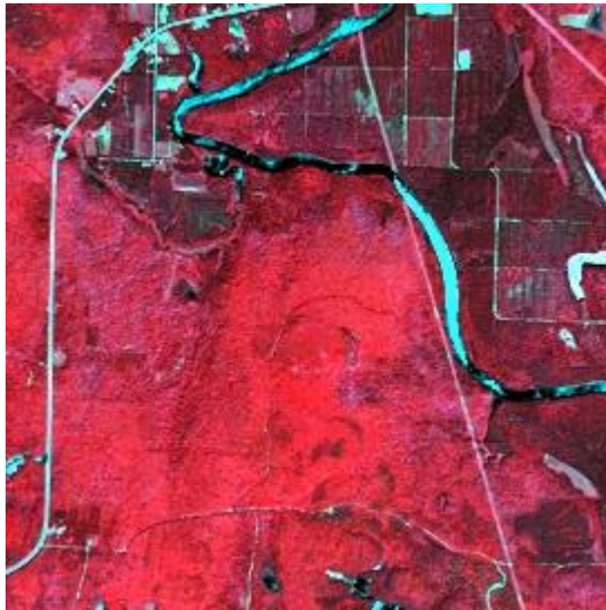
Figure 3.7. False colour composite of resampled Quickbird Image. Quickbird band 2 set to blue, band 3 set to green, band 4 red.
