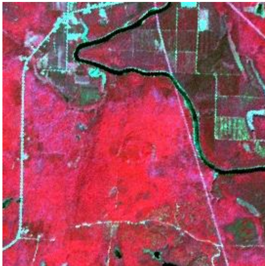
Figure 3.6. False colour composite of the ASTER study area. ASTER band 1 set blue, band 2 set as green, and band 3 set as red.
