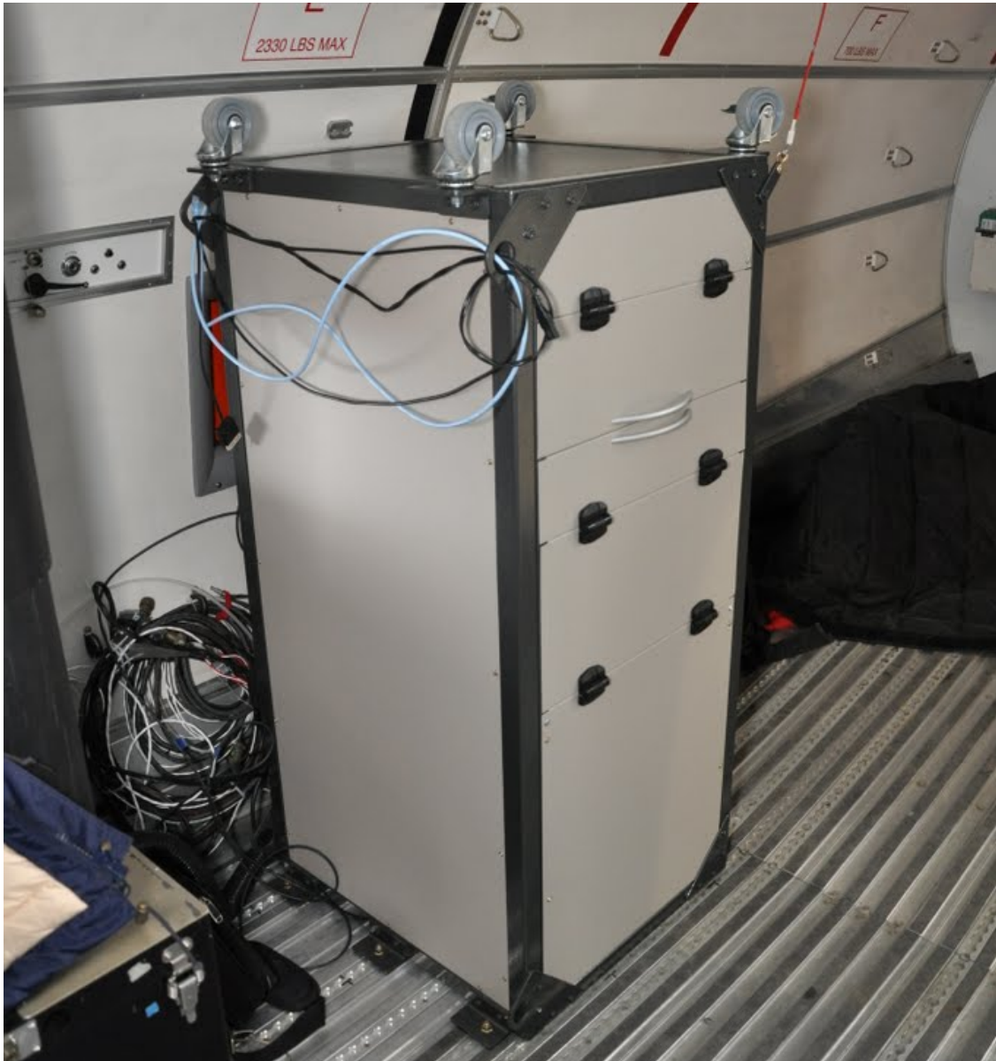
Figure 4.2: The DIAL installed aboard the Polar 5. The lidar is contained in the aircraft rack bolted to the seat tracks.
