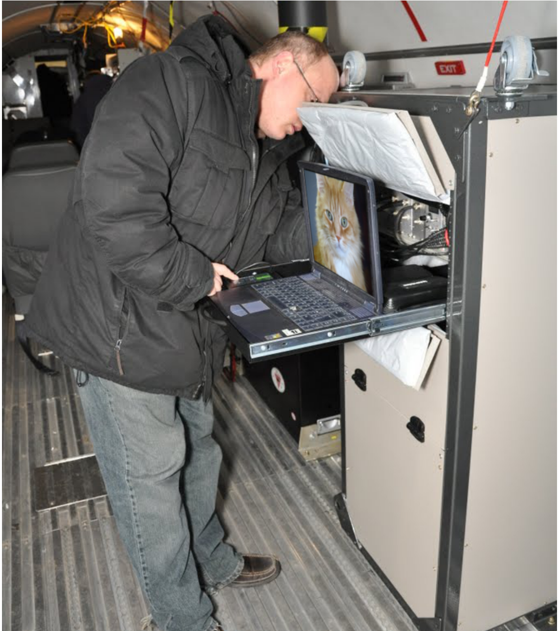
Figure 4.3: The DIAL installed aboard the Polar 5. Hinged panels allow access to the Licel electronics and data logging PC.
