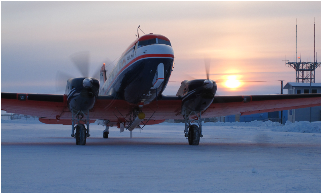
Figure 4.1: The Polar 5 research aircraft. Basler BT-67: rebuilt and modernized DC-3
