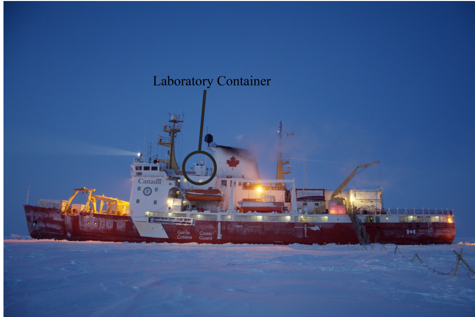
(a) Amundsen Icebreaker Ship. The laboratory container (circled) is located on the top deck between the bridge and smoke stack.
