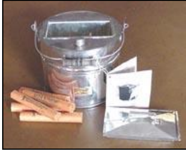
Figure 2.7 A commercial dynamite thawer. Cartridges were inserted into the opening and warm water circulated around them.
