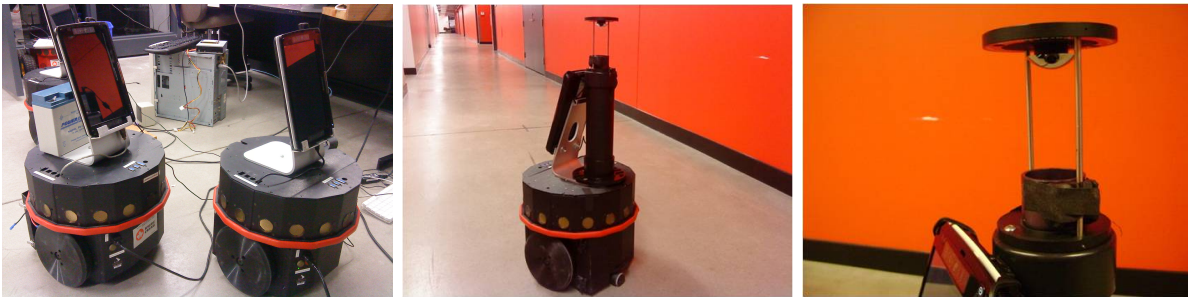
(a) original super-scout robots in VGR lab. (b) super-scout robot augmented with an omni-directional vision sensor. (c) spherical mirror of the vision sensor.
