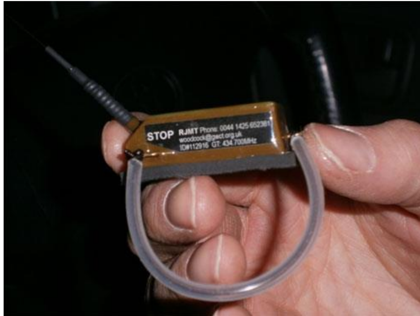
Figure 4: Platform Transmitter Terminal (PPT) Device that Attaches to a Bird [16]
