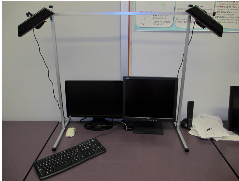
Figure 1-2: Picture of the 3 Gear System setup. Two Kinect™ cameras on either side of metal frame track hands operating in the space above the desk.
