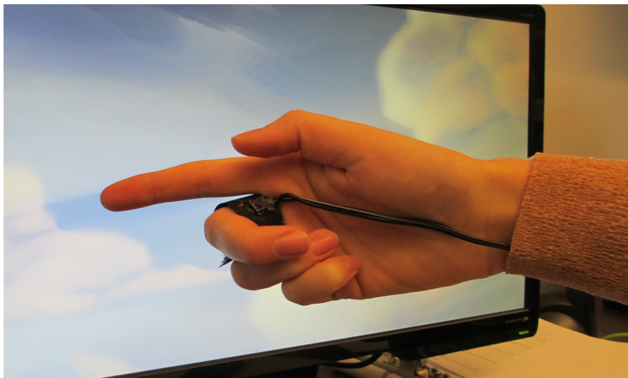
Figure 3-8: Photo of finger ring with the button visible below the users thumb (raised more than normal for illustration). Self adhesive tape was used to keep the cable from interfering with user motions.
