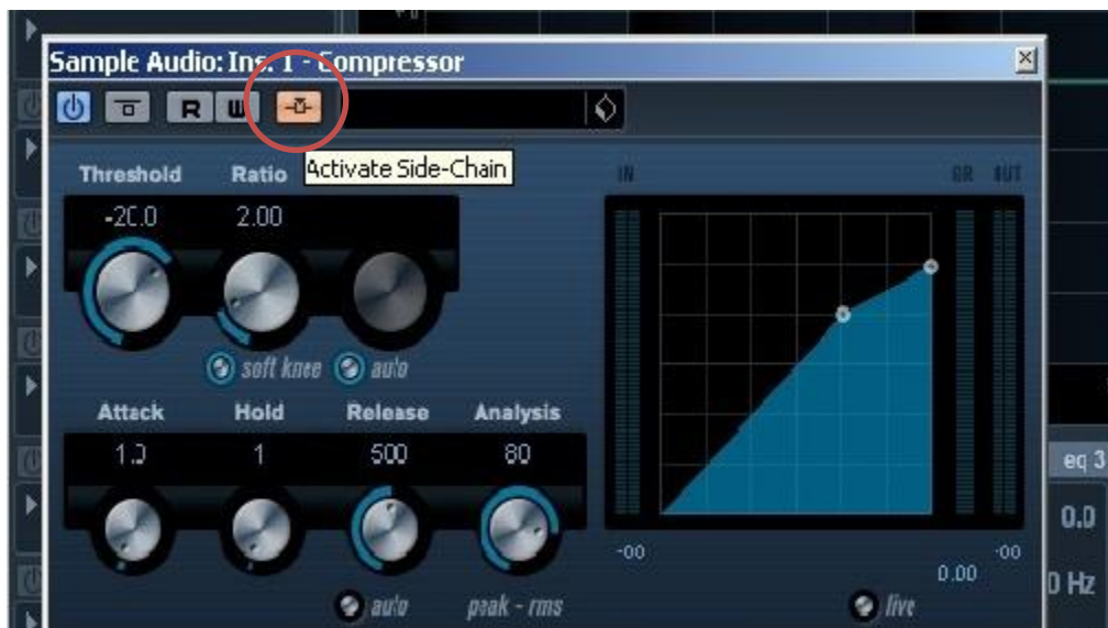
Figure 43: Cubase DAW compressor with sidechain input activated
