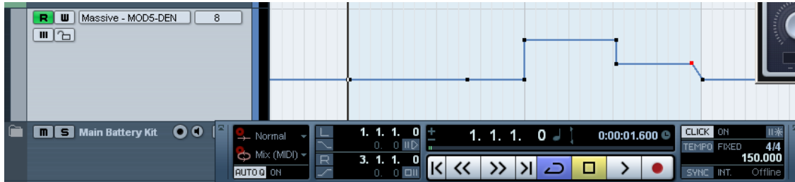
Figure 45: Cubase DAW automation curve mapped to Massive's LFO5 rate
