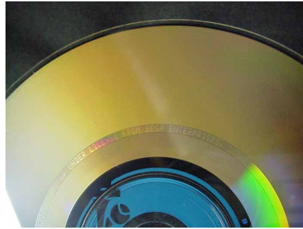
Figure 6. A view of the dual layers within a Dreamcast GD-ROM disc (Sega Enterprises, Inc)
