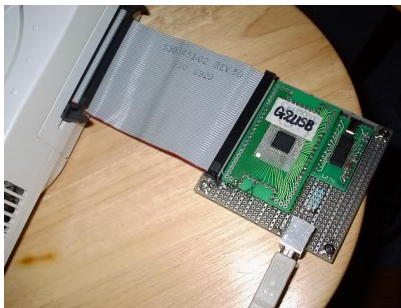
Figure 9. Custom made Broad Band Adaptor for the Dreamcast, jj1om.
