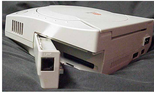
Figure 4. The Dreamcast Modem, partially removed from the console.
