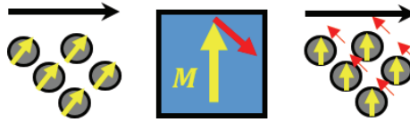
Figure 5: Schematic of the origin of spin-transfer torques (STTs) in FM metals. The yellow arrows represent the direction of the magnetic moment.
