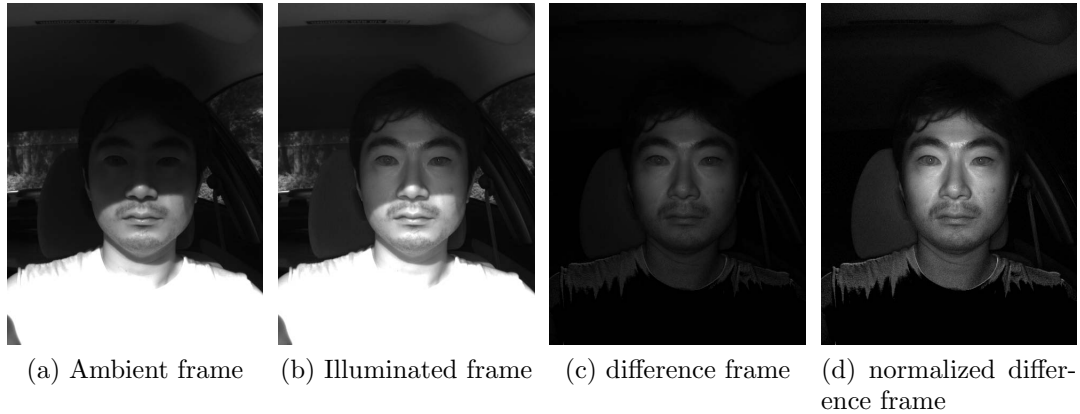
Figure 13: Example ambient, illuminated and difference frames are shown. Only the image in (d) was normalized to be visualized in proper contrast.
