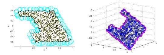
(a) Boundary extracted on the projected 2D  $\,$  (b) Boundary back-projected to 3D space point set
