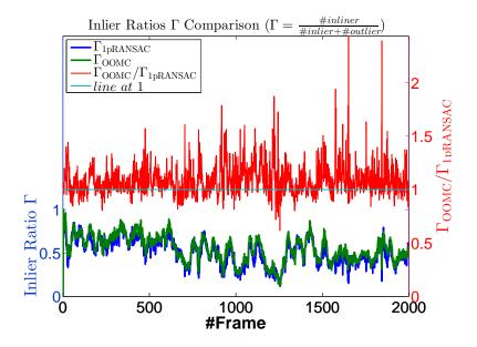
**Figure 19:** Inlier ratios of 1pRANSAC algorithm and OOMC algorithm, and their comparison. The inlier ratios are from the maximum support consensus sets for each frame.
