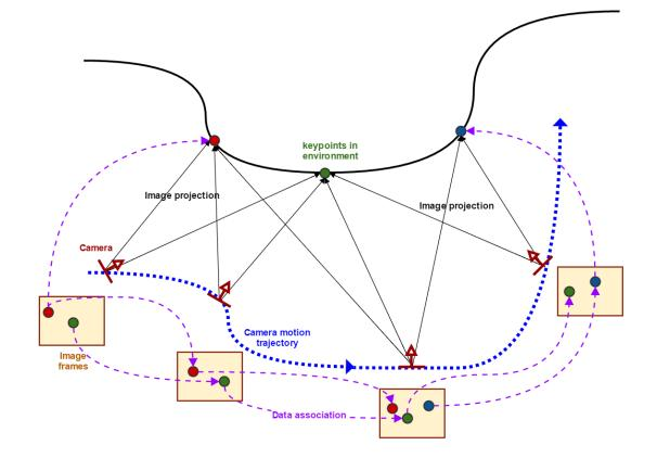
**Figure 2:** An illustration of the dynamics and measurements process involved in the VSLAM problem.
