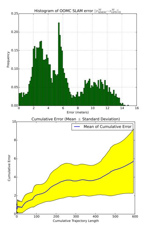
**Figure 23:** Errors of OOMC SLAM compared to the GPS ground truth. Top: histogram of instantaneous error. Bottom: cumulative errors with  $1-\sigma$  range along the trajectory.
