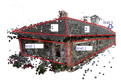
Figure 52: Planes measured using total stations to provide ground truth data.
