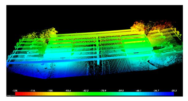
Figure 10: A PCD of a bridge, captured by a profession total station.
