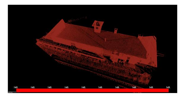
Figure 11: A PCD of a building, generated using VSLAM techniques.
