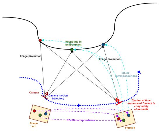
Figure 12: VSLAM system completely observable condition #1.
