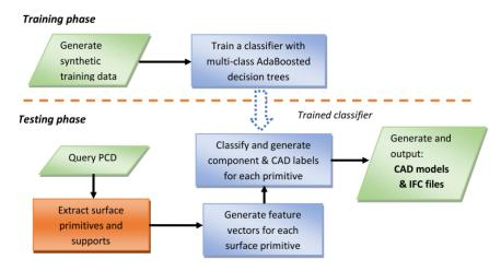
**Figure 54:** Pipeline of the algorithm for semantic recognition of PCDs based on Surface Primitives.
