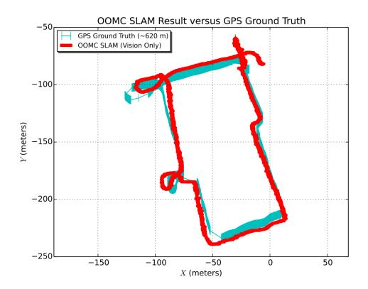
**Figure 22:** Estimated trajectory from the OOMC SLAM compared to trajectory from a RTK Differential GPS.
