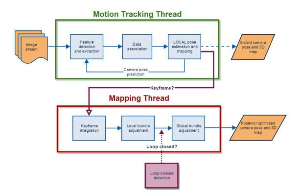
Figure 7: A typical design of a keyframe based bundle adjustment VSLAM system.
