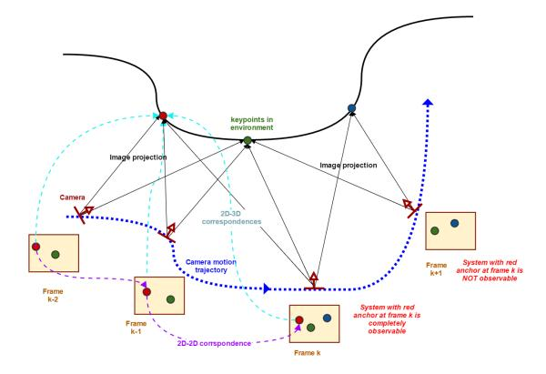
Figure 13: VSLAM system completely observable condition #2.
