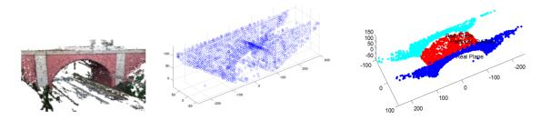
**Figure 55:** Results of surface primitive modeling. Left: input PCD. Middle: down-sampled PCD. Right: detection and classification results.
