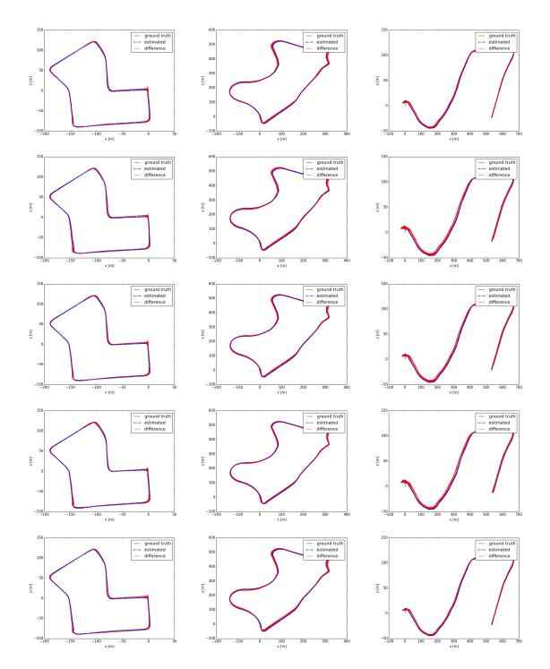
**Figure 37:** Results on original KITTI 07, 09, and 10: estimated trajectory, ground truth, and translation errors. Row 1: 20% GFs. Row 2: 30% GFs. Row 3: 40% GFs. Row 4: 50% GFs. Row 5: 60% GFs. Note that the X and Z axes are of different unit lengths, for better illustration of localization error.
