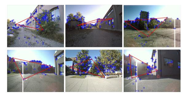
**Figure 21:** Example frames from 620m sequence. The detected features are plotted in blue circles and the selected triplets are plotted in red triangles.
