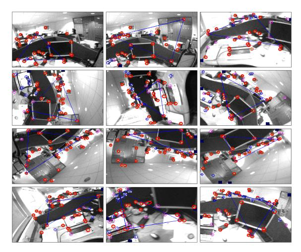
**Figure 15:** The triplets (depicted as blue triangles) selected for EKF update in example frames from the 1pRANSAC dataset. The measurements are plotted in eclipses of  $1-\sigma$  regions with various markers: thick red – low-innovation inliers; thin red – high-innovation inliers; magenta: rejected spurious matches; blue – no match found by cross-correlation.
