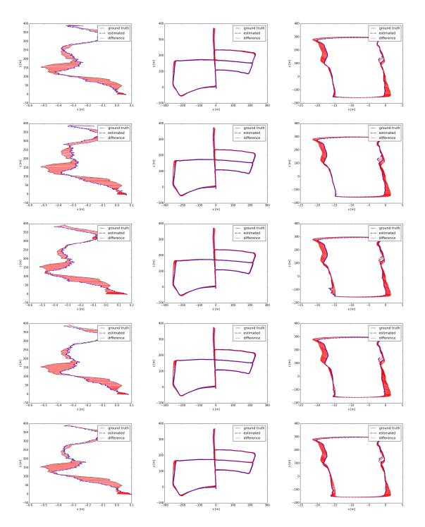
**Figure 36:** Results on original KITTI 04, 05, and 06: estimated trajectory, ground truth, and translation errors. Row 1: 20% GFs. Row 2: 30% GFs. Row 3: 40% GFs. Row 4: 50% GFs. Row 5: 60% GFs. Note that the X and Z axes are of different unit lengths, for better illustration of localization error.
