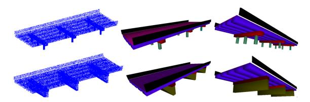
**Figure 56:** Left: query PCDs. Middle and right: augmented models consisting of a collection of CAD entities colored by semantic labels.
