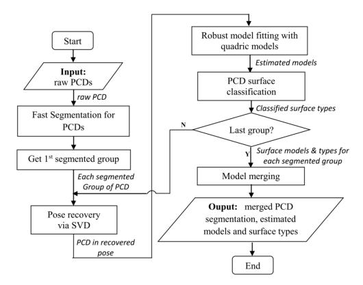
Figure 53: Flowchart of the surface primitive-based PCD modeling algorithm.
