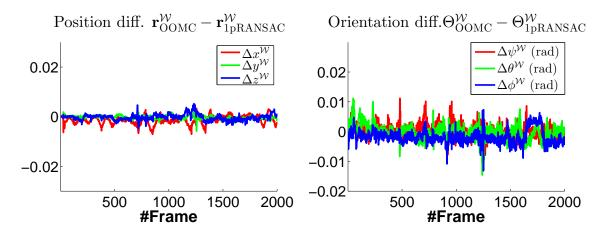
**Figure 17:** Differences in camera localization results of 1pRANSAC SLAM and OOMC SLAM
