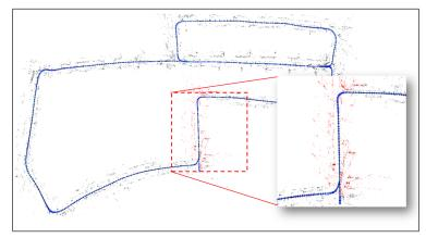
(c) Original ORB-SLAM: Estimated trajectory of sequence 05 at 243 sec, after loop-closure.
