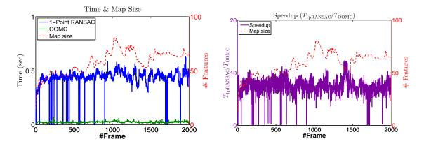
**Figure 18:** Left: execution time of 1pRANSAC and OOMC, and the map size. Right: speedup of OOMC over 1-Point RANSAC.
