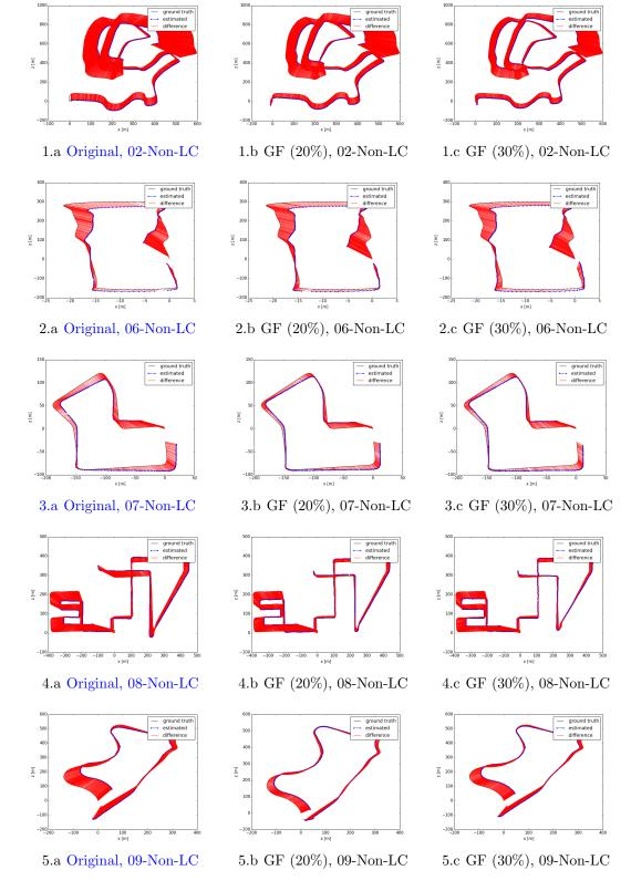
**Figure 40:** (Continued in Figure 41.) Estimated trajectory, ground truth, and translation errors on none-loop-closure sequences. Note that the X and Z axes are of different unit lengths, for better illustration of localization error.
