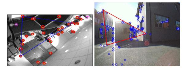
**Figure 14:** At each time segment, the OOMC algorithm identifies the feature triplet (defines the triangles) which forms the subsystem of **optimal observability** and **minimal cardinality** with the camera state. Localization and mapping is then performed with this subsystem.
