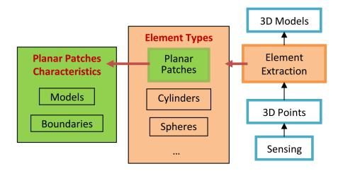
**Figure 42:** Role of planar patches extraction in the automatic conversion from raw PCDs to 3D models.
