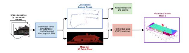
**Figure 1:** The pipeline of the solution to 3D modeling from image sequence. The whole pipeline is composed of two key components: monocular visual simultaneous localization and mapping, and point cloud data modeling.
