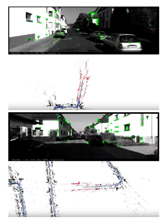
**Figure 33:** Two examples of the keyframe BA VSLAM system in action, on the KITTI dataset. In each sub-figure, top: current frame plotted with tracked visual features; bottom: estimated camera trajectory and 3D positions of the features.
