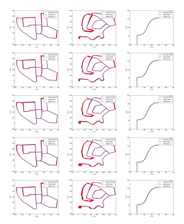
**Figure 35:** Results on original KITTI 00, 02, and 03: estimated trajectory, ground truth, and translation errors. Row 1: 20% GFs. Row 2: 30% GFs. Row 3: 40% GFs. Row 4: 50% GFs. Row 5: 60% GFs. Note that the X and Z axes are of different unit lengths, for better illustration of localization error.
