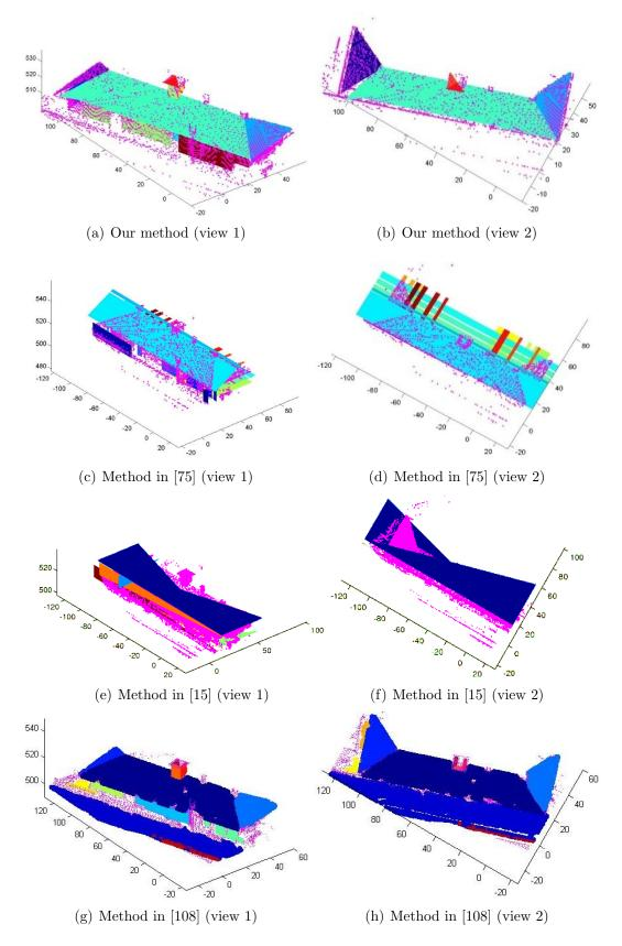
**Figure 51:** Extracted planar patches for the building PCD using different methods, plotted with the raw PCD (in magenta).
