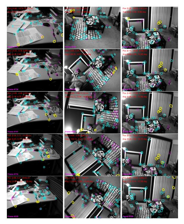
**Figure 30:** Example frames from data-association experiment. The strongly observable features are illustrated in yellow, retrieved inlier set is in cyan, and the outlier set is in purple. Column 1: camera is moving away from the desktop. Column 2: camera is rotating w.r.t. the optical axis. Column 3: camera is rotating w.r.t. the x axis of camera.
