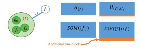
**Figure 25:** In spatial grouping, selecting one more feature as anchor results in an additional row-block in the measurement Jacobian, which further expands the SOM.
