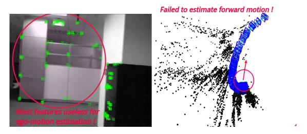
**Figure 9:** An example showing that not all the features contribute in the same level to the localization accuracy. Left: features detected and tracked in the current frame. Right: the incorrect camera trajectory estimated.
