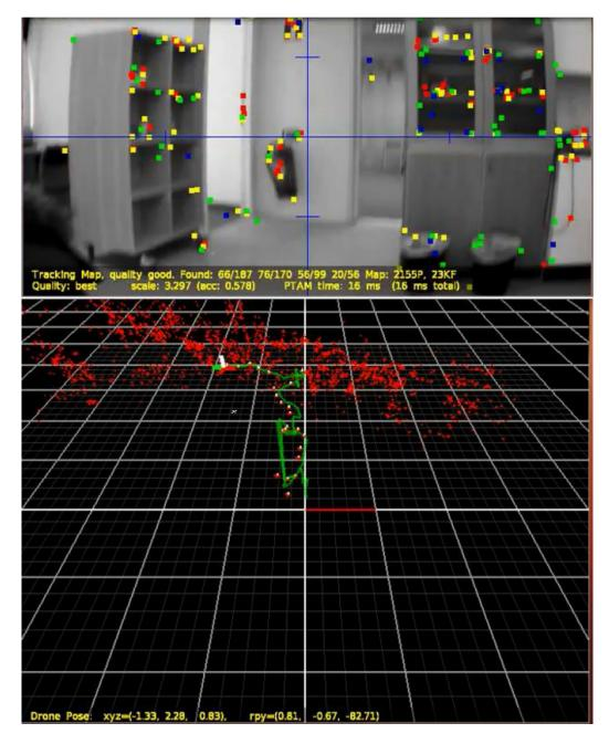
**Figure 8:** An example of keyframe based BA VSLAM: PTAM (parallel tracking and mapping) system [60]. Top: current frame plotted with tracked visual features. Bottom: estimated camera trajectory and 3D positions of the features.
