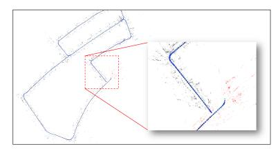
(a) Original ORB-SLAM: Estimated trajectory of sequence 05 at 241 sec, before loop-closure.
