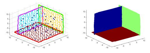
(a) Detected boundaries of extracted planes (b) Final planar patches representation
