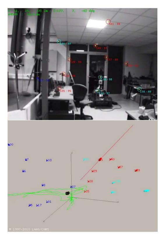
**Figure 6:** An example of EKF-VSLAM: RT-SLAM system [81]. Top: current frame plotted with tracked visual features. Bottom: estimated camera trajectory and 3D positions of the features.
