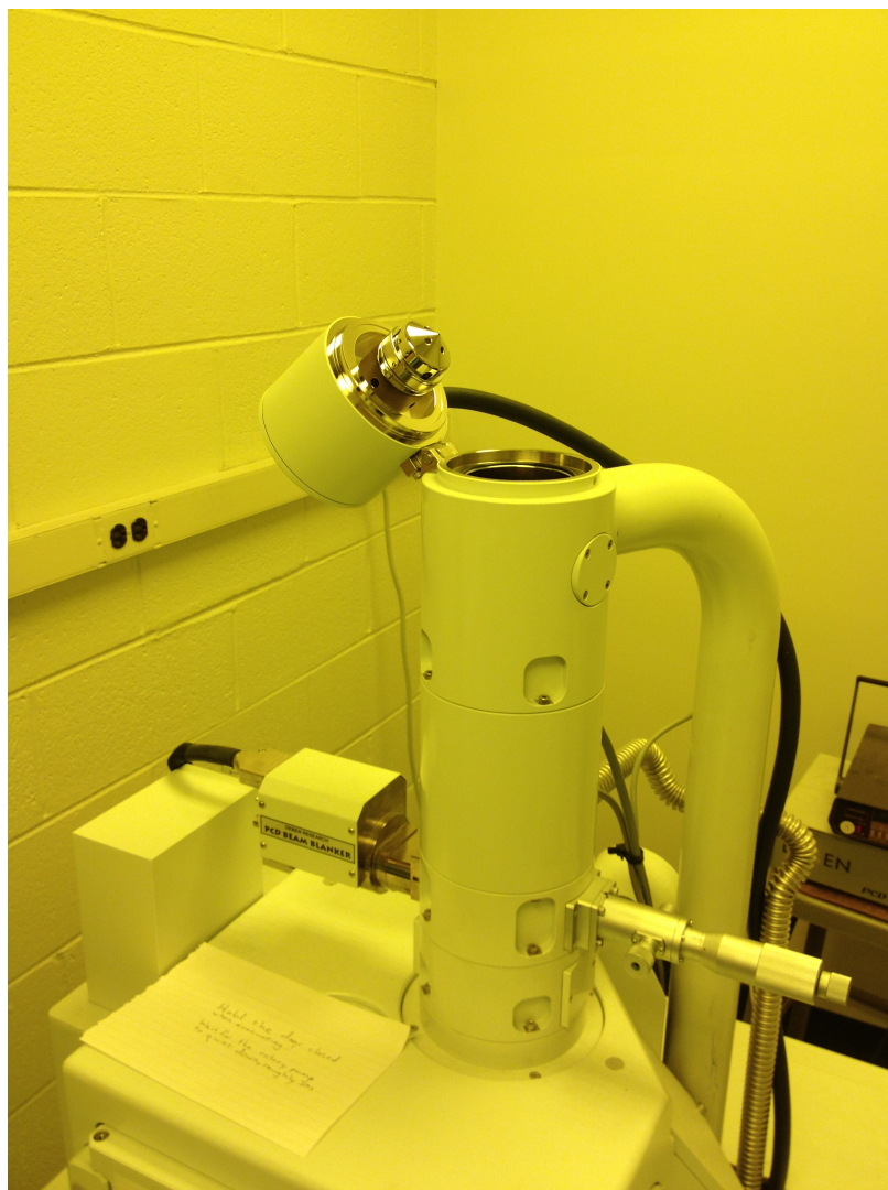
Figure 2.2: Photograph of Scanning Electron Microscope that I use to image samples and conduct electron-beam lithography. Optical column is open at the top during a routine filament replacement. The silver cone is the wehnelt.
