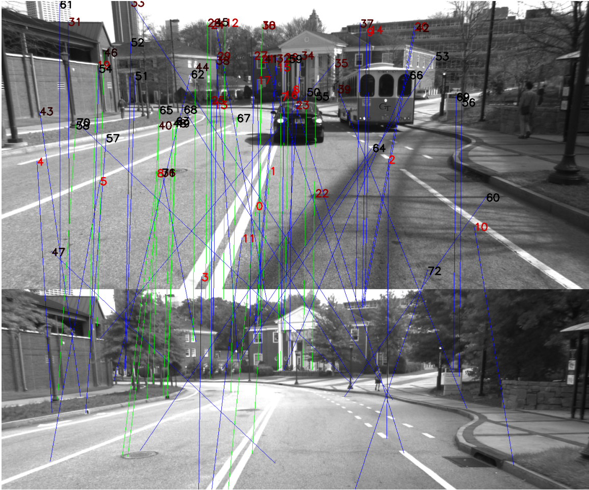
Figure 21: Successful loop closure and pose recovery on challenging imagery between frames from sequences K (top) and L (bottom). There are notable differences in lighting, foliage, as well as vehicular occlusions. Putative matches are shown in blue, and accepted inlier matches are shown in green.
