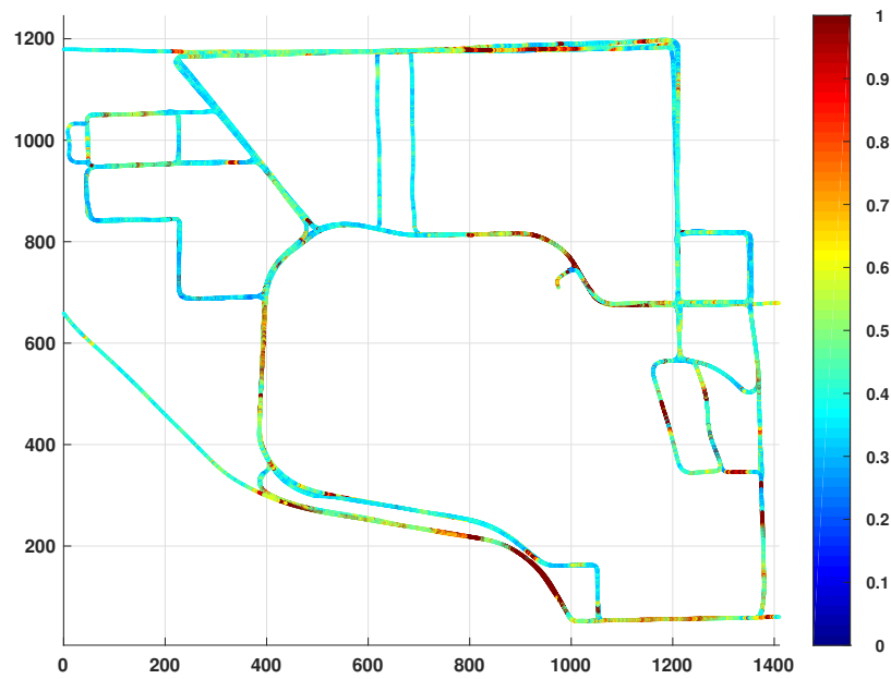
Figure 28: Root mean square projection errors per camera for the fully optimized Submap-STM.
