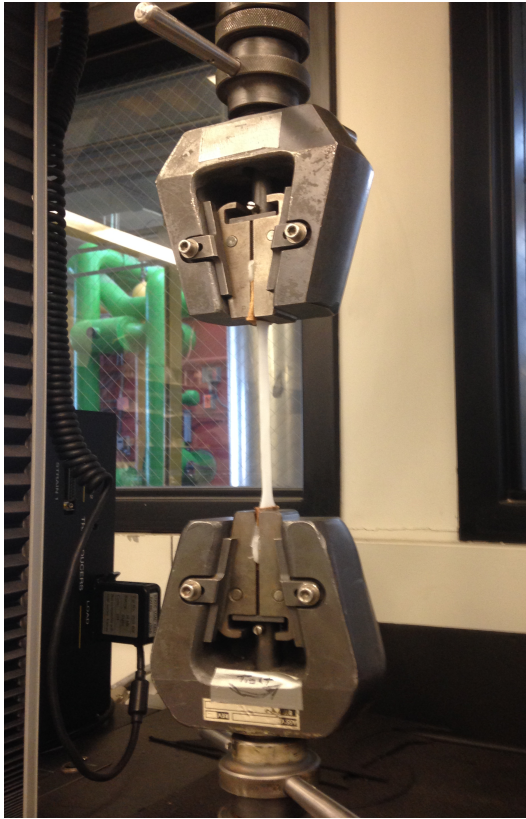
Figure 20: Display of extensometer test for tensile strength
