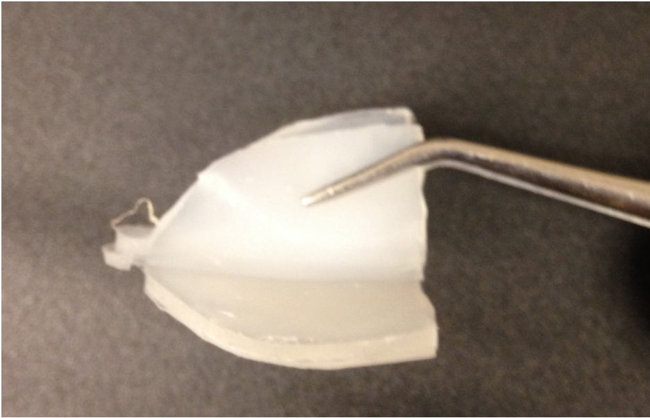
Figure 13: example of lab-fabricated PVA palatal obturator
