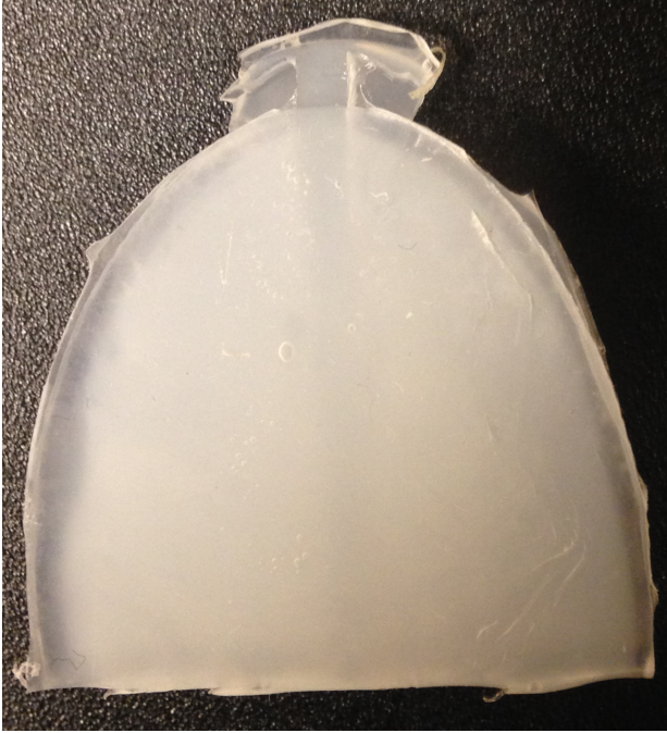
Figure 15: example of lab-fabricated PVA palatal obturator (sample cut out manually with surgical scissors, hence ragged edge)
