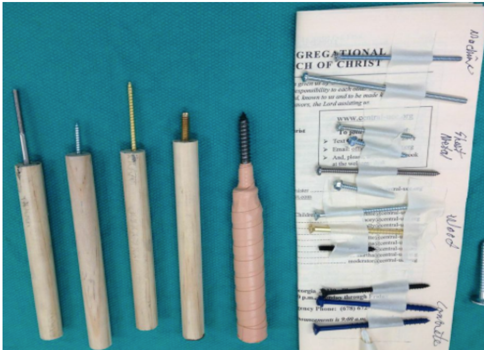
Figure 50: Set of industrial screws used for cadaver testing (dilation of implant pocket)
