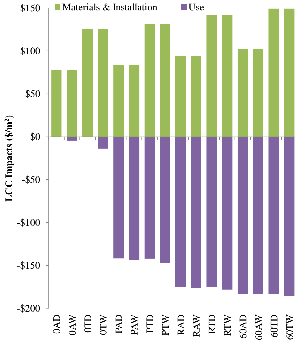
Figure 4.10: LCC results of roofing options in Atlanta when retrofitting from no insulation.
