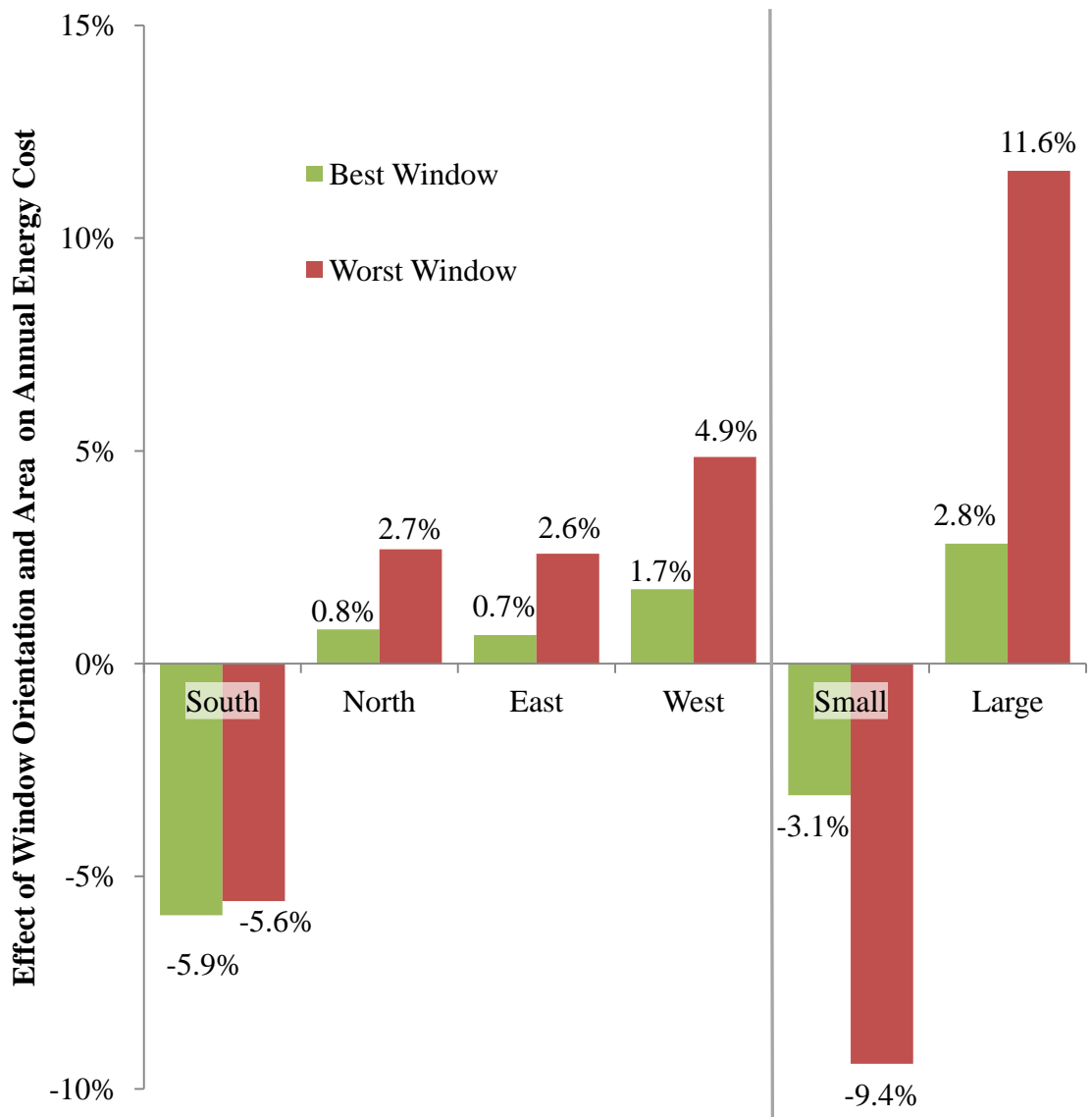
Figure 3.4: The effect of orientation (compared to equal orientation) and window area (compared to a medium 15% WWR) on the annual energy cost of the home.
