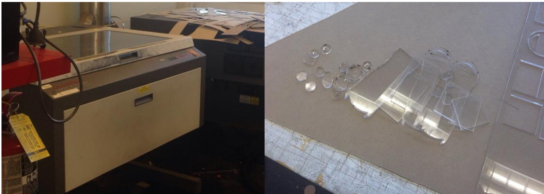
Figure 22. Process using laser cutting to fabricate the mini-flashlight model
