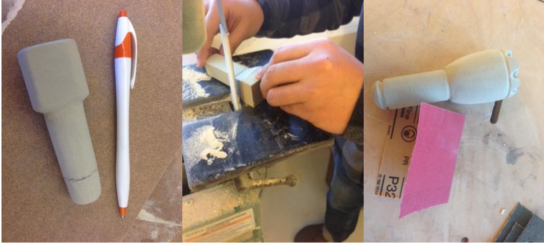
Figure 26. Process of making handmade mini-flashlight model
