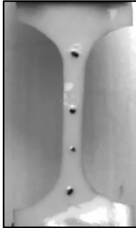
Figure 1. Image of dog-bone shaped sample with four markers
