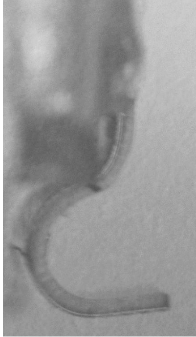
Figure 50: Side View of Failed Plated Spring after 18 Million Cycles at 4x Magnification
