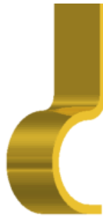
Figure 21: Rendering of the Modified Spring Design for Side Mounting
