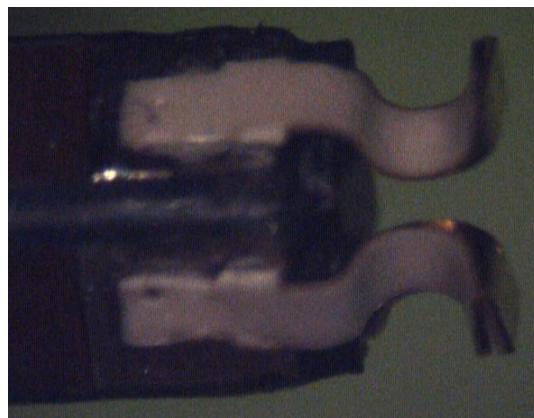
Figure 39: Interconnect Prototype with Individually Installed Springs
