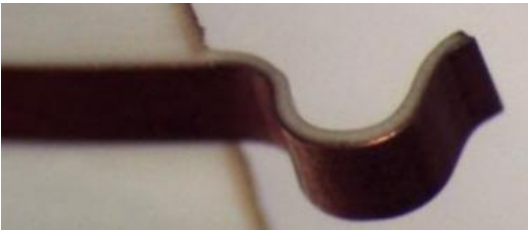
Figure 35: LCP Spring Formed With Hybrid Mold Using a 0.028" Gauge Pin
