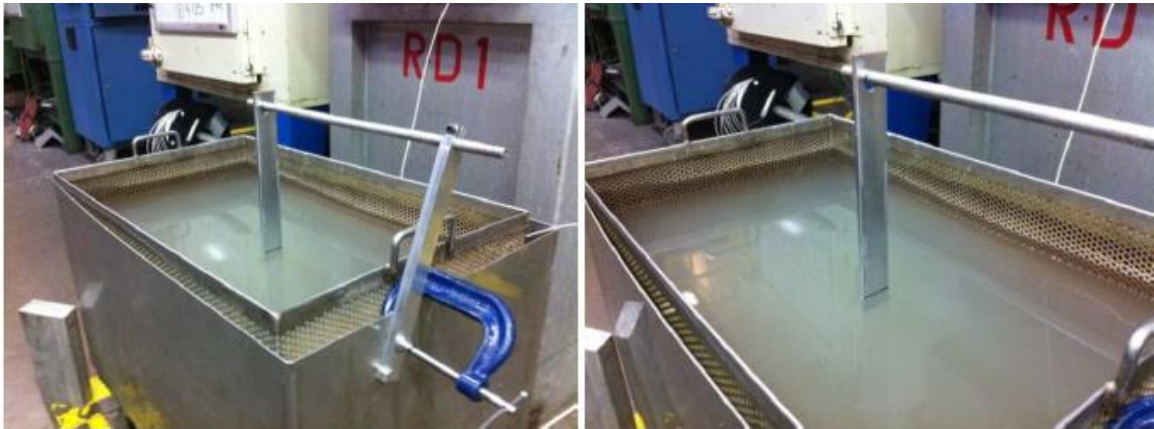
Figure 163 – Quench rate test set-up. The sample is 30.48 cm (12 in) long with 3.81 cm (1.5 in) submerged below the water line. It was held in the circulated quench tank for 10 minutes before being fully quenched.
