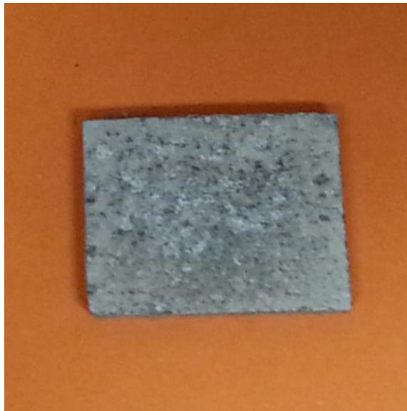
Figure 260 – GT6-T73 after 48 hours in EXCO solution.
