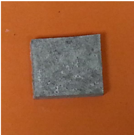
Figure 257 – GT3-T73 after 48 hours in EXCO solution.
