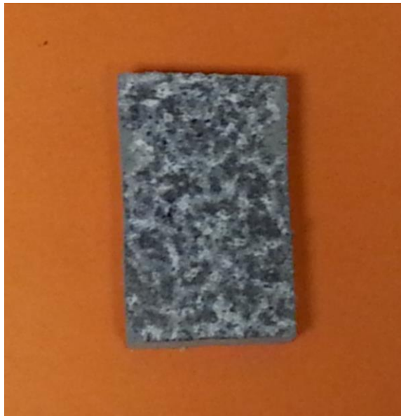
Figure 255 – GT1-T73 after 48 hours in EXCO solution.
