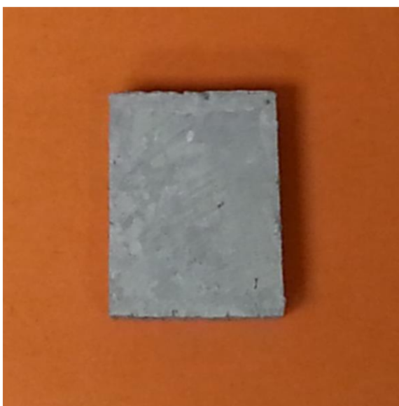
Figure 259 – GT5-T73 after 48 hours in EXCO solution.
