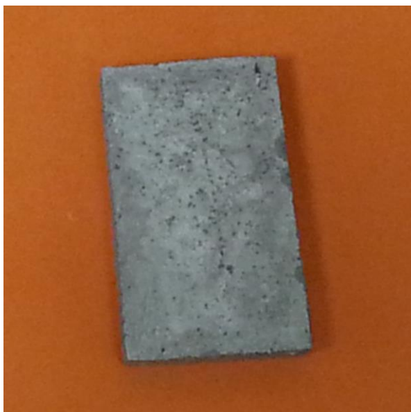
Figure 258 – GT4-T73 after 48 hours in EXCO solution.
