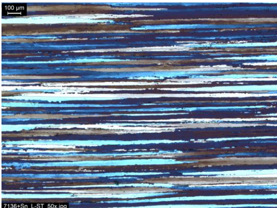
Figure 158 – 7136+Sn bar L-S (Barker's Reagent).
