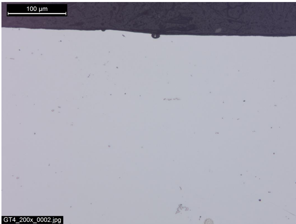
Figure 267 – A typical IGC attack on GT4-T73 at 200x.
