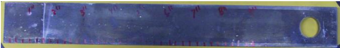
Figure 155 – Example of a quench test sample (7136, W-temper).
