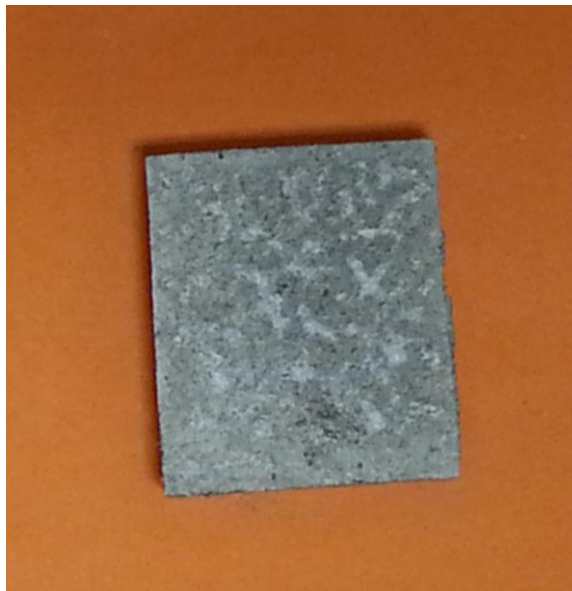
Figure 261 – GT7-T73 after 48 hours in EXCO solution.
