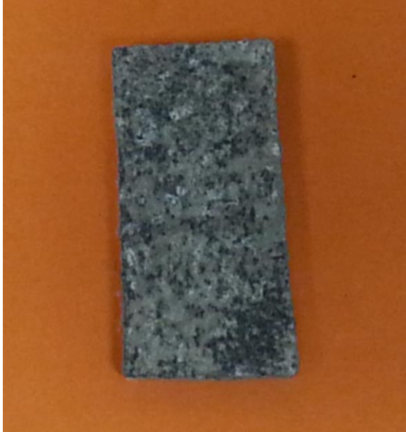
Figure 256 – GT2-T73 after 48 hours in EXCO solution.
