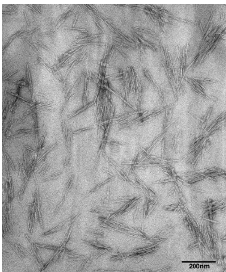
Figure 2.1: TEM of wood derived CNCs.
