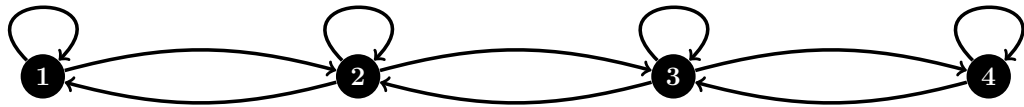
(a) An example of a 4 node interaction exchange graph. The arrows pointing into a particular node indicate what information is able to be received by that particular agent.
