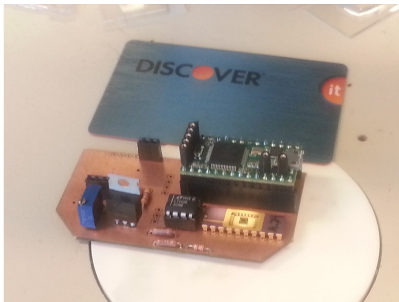
Figure 6.14: Final portable integrated device, including interface electronics, sensor packaging and telemetry modules. Its overall size is smaller than a credit card in length and width.
