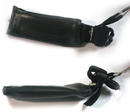
Fig. 25 Pneumatic sensor from front ( top ) and from side ( bottom )
