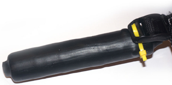
Fig. 21 Capacitive sensor in heat shrink tubing
