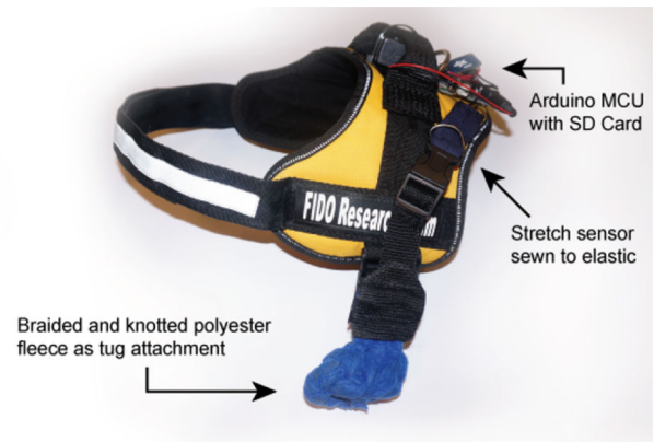
Fig. 11 Revised tug sensor on vest
