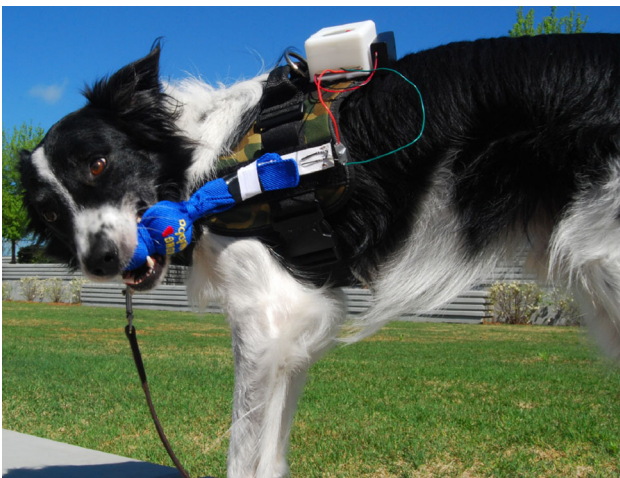
Fig. 8 Border collie activating tug sensor on-body
