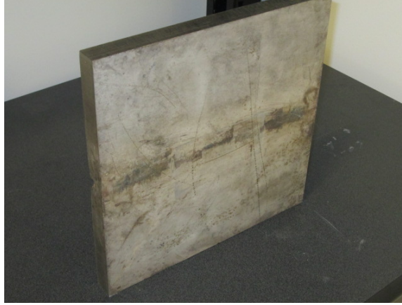
Figure 14: 12"x12"x1" 304 stainless steel plate used for weld sensitization measurements
