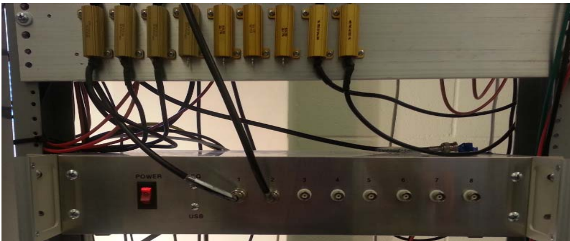
Figure 8.6: National Instrument data acquisition unit (bottom) with scaling resistors (top).
