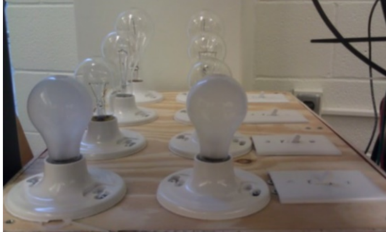
Figure D.4: Photograph of single-phase load.
