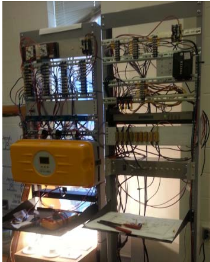
Figure 8.1: Laboratory setup for PV array fault analysis.
