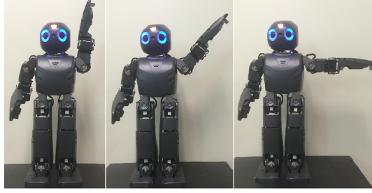
Figure 41: DARwIn-OP is used as the humanoid robotic platform in this study. Image shows snapshots of Darwin performing the nonverbal gestures.
