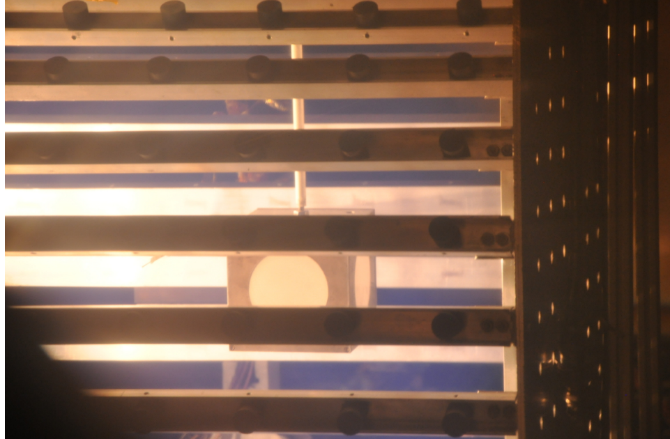
Figure 9.3: Photo of plasma cell testing at 500 mA discharge current with grooved and non-grooved BN samples. Argon plasma, pressure = 1 \times 10^{-4} Torr-Ar.
