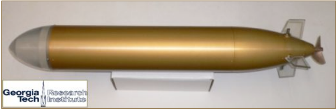
Figure 14: Yellowfin Autonomous Underwater Vehicle - designed to be man-portable for oceanographic observation.
