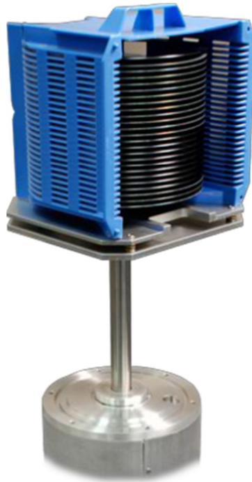
Figure 1.8: Elevator mechanism. Elevator mechanism used in load-lock to drive wafers vertically, reducing or eliminating the requirement for vertical motion in the vacuum robot. Photo courtesy of Genmark Automation, Inc.
