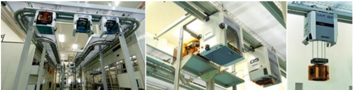
Figure 1.4: OHT moves FOUPS between process steps. Left: Multiple OHT vehicles move along an overhead track between process steps. Center: A FOUP is loaded onto an OHT vehicle. Right: A FOUP is lowered from an OHT vehicle using a belt hoist system. Photos Courtesy of Daifuku Co, Ltd.
