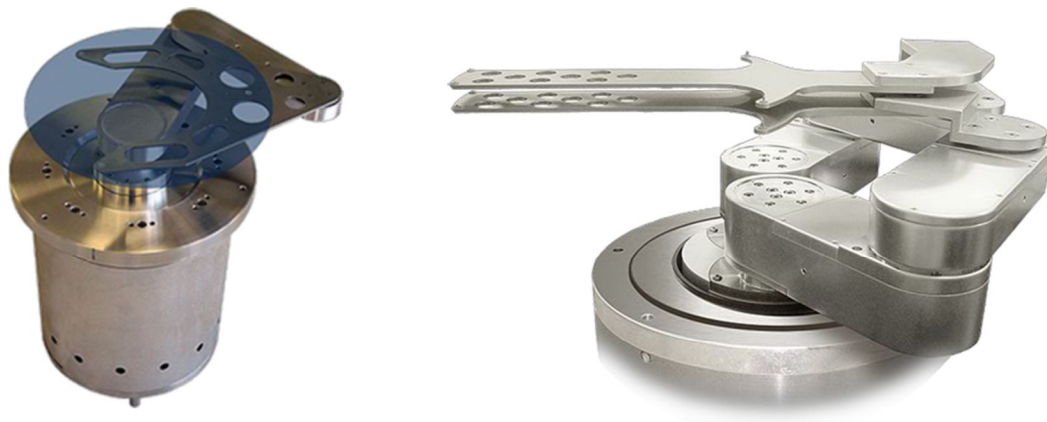
Figure 1.7: Two examples of vacuum robot architecture. Left: Vacuum robot with base rotate axis and belt-driven extend axis. Right: Dual end-effector robot with both arms retracted. Robot consists of 6 motion axes: rotary and linear axes at the base, a belt-driven rotary extension axis for each arm set, and a linear axis for each end effector. Photos courtesy of Genmark Automation, Inc.
