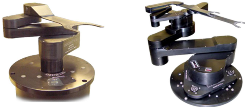
Figure 1.5: Two examples of atmospheric robot architecture. Left: Single end-effector atmospheric robot comprised of 2 rotary axes (a rotation at the base and a belt-driven extension) and a vertical linear axis requires a horizontal track to feed multiple load ports. Right: Dual end-effector atmospheric robot with 8 motion axes can feed four load ports without a track. Robot has a vertical linear axis at the base, a rotary axis at the base, a belt-driven extend axis, a rotary axis to allow rotation of the third link, and rotary and linear axes on each end effector. Images Courtesy of Genmark Automation, Inc.
