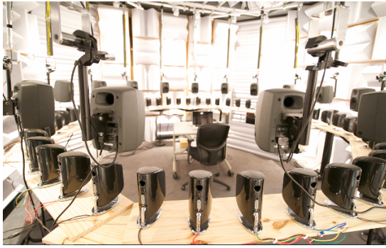
Figure 1: Experimental setup in the CIRMMT Spatial Audio Lab. Both loudspeaker arrays consist of equally spaced loudspeakers on a 3.5-m circle in the horizontal plane (16 Genelec for the top one, 48 B & W for the bottom one).
