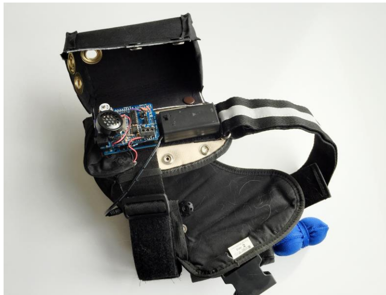
Fig. 11. Prototype 4 used a large fabric box secured with snaps to house the Arduino UNO, its wave shield, and the speaker. We used screw terminals to secure the wires in case the interface needed to be replaced.
