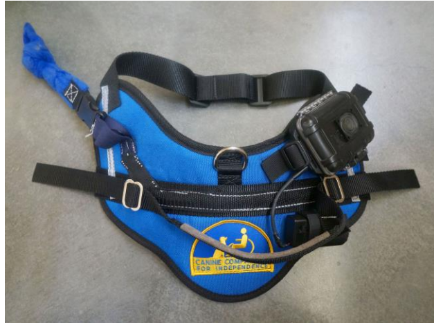
Fig. 7. Prototype 2 used an official service dog harness. This design concealed the wires and electronic components to achieve a simpler look.
