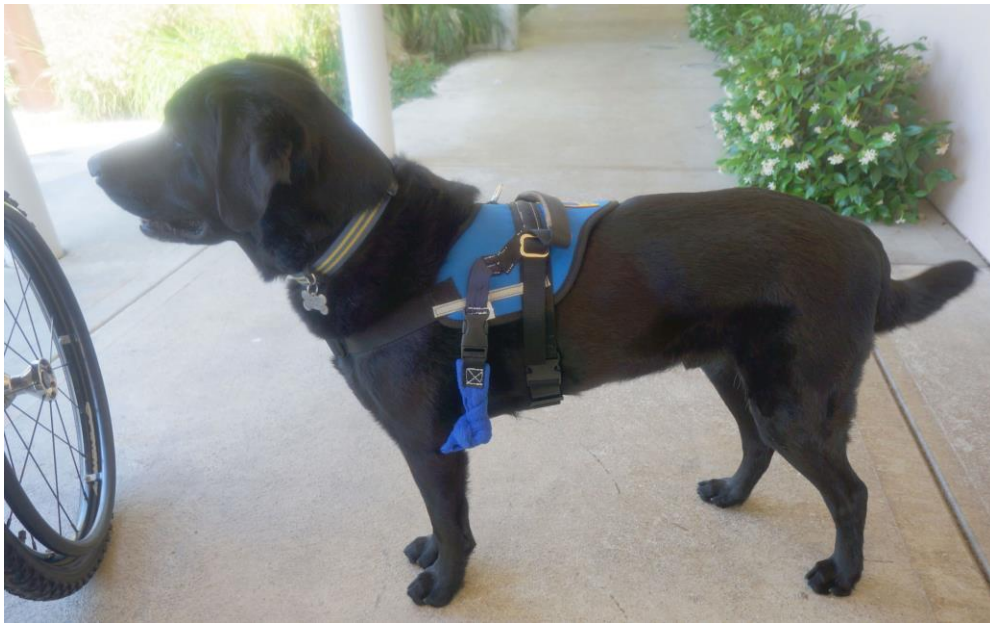
Fig. 2. A service dog wears one of the early prototypes. When tugged, the microcontroller on the harness plays a message saying “ My owner needs your attention, please follow me! ”
