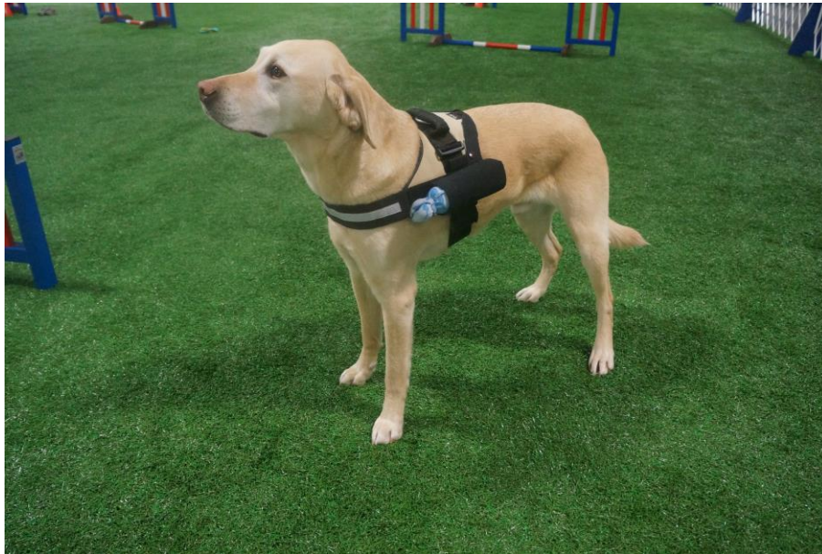
Fig. 10. Prototype 3 being worn by one of the participants. This prototype has a fabric tube that holds the tug affordance in place. The tube can be angled downwards to provide easier reach.
