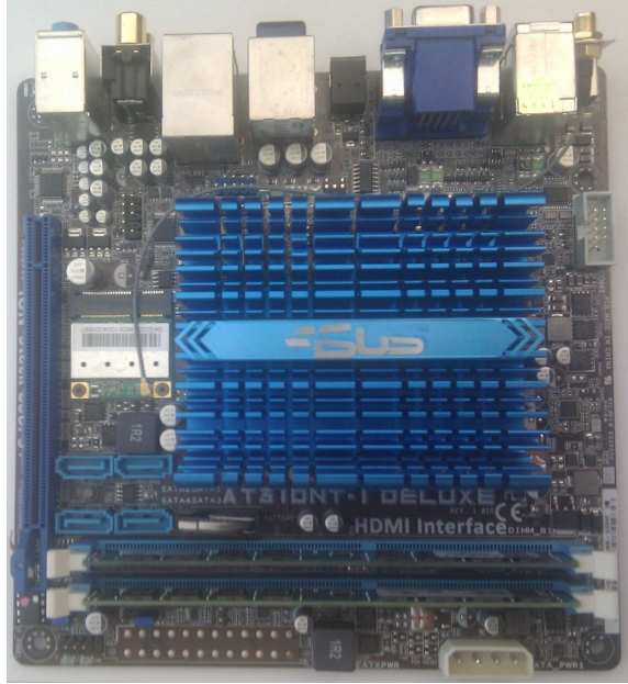
Figure 32: Asus AT3IONT-I NVIDIA ION GPU platform
