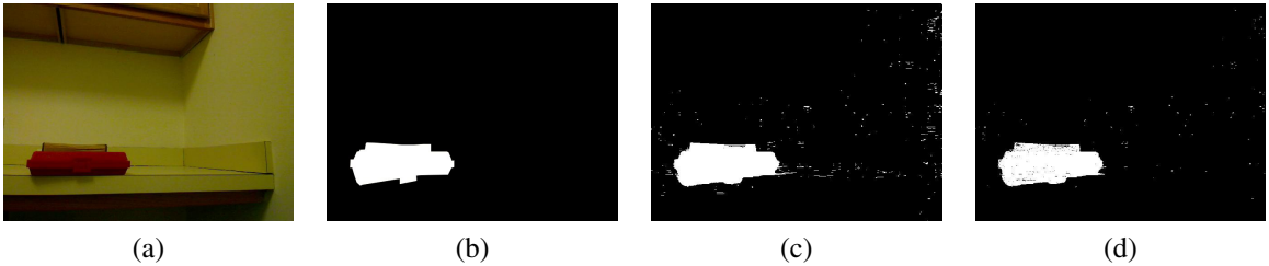
Figure 21: Indoor boxes, filtering at 50% observability threshold: (a) Original image (b) Ground truth (c) Unfiltered (d) Filtered
