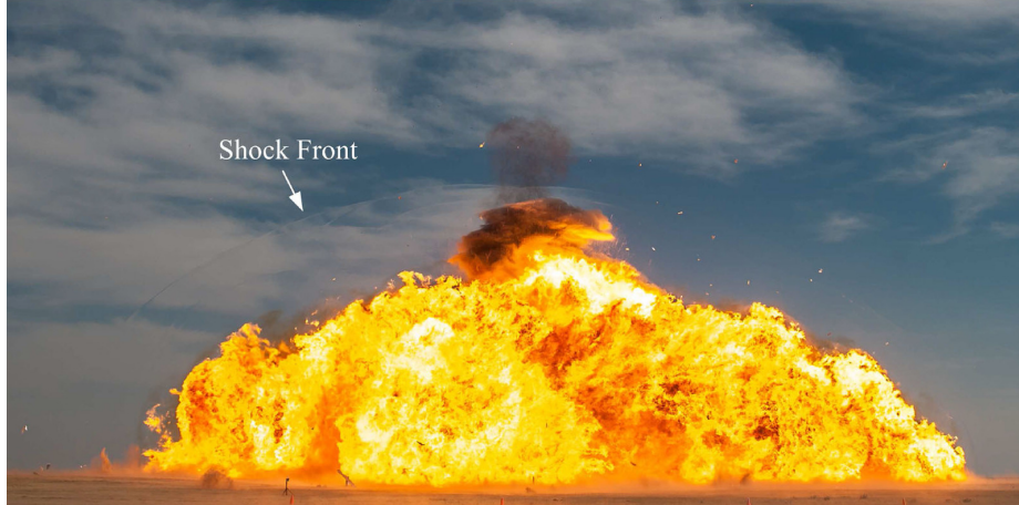
Figure 5: Blast wave and fireball formed after detonation of gasoline spray cloud [132]. Reprinted with kind permission from Springer Science and Business Media (Figure 3 from Zhang et al., Shock Waves , 25, 239-254, 2014; Copyright 2014, Springer)
