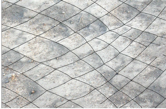
Figure 1: Cellular structures recorded on the ground by a gasoline spray detonation [132]. Reprinted with kind permission from Springer Science and Business Media (Figure 7 from Zhang et al., Shock Waves , 25, 239-254, 2014; Copyright 2014, Springer)
