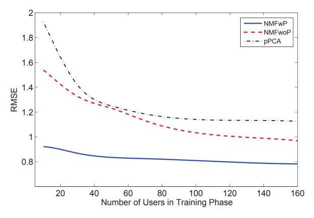
**Figure 20:** The average RMSEs of the three prefix based algorithms with different number of simulated players for training.
