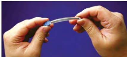
Figure 65: Bending a flex sensor
