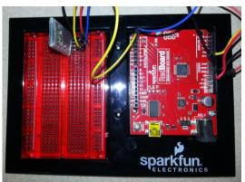
Figure 2. Electronics integrated with Hand Mentor device.
