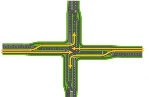
Figure 22. Continuous Flow Intersection Diagram. Source: Compass
