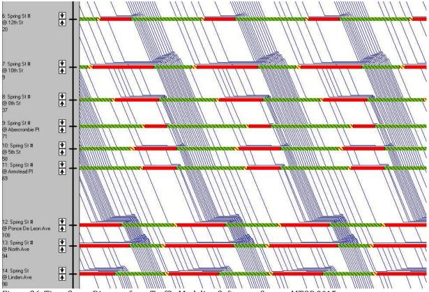
Figure 26. Time-Space Diagram from Traffic Modeling Software. Source: MTOP 2015
