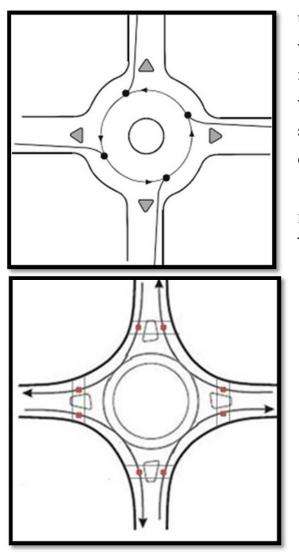
traffic flow becomes an impediment (an issue with any intersection). Additionally the roundabout is designed with a consolidated vehicle path so the number of conflict points is significantly reduced to only 4 vehicle to vehicle conflict points and 8 vehicle to pedestrian points.
