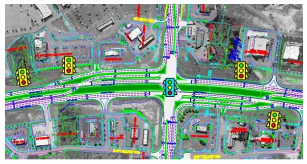
Figure 35. Dawsonville CFI VISSIM model with turning movements added. Source: GS&P
