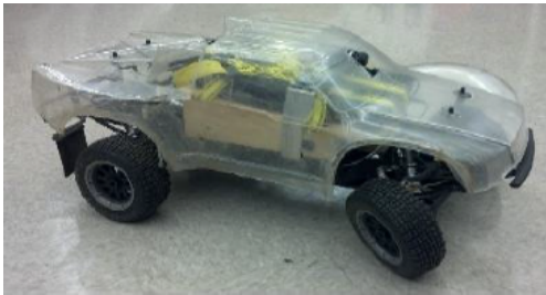
Fig. 3: Our platform is a high-speed mobile robot, a modified 1/8 -scale radio-controlled car approximately 50 cm in length with on-board sensors and computing. The camera has a high-distortion 110^\circ FOV lens. The robot was operated at approximately 2m/s during data collection.
