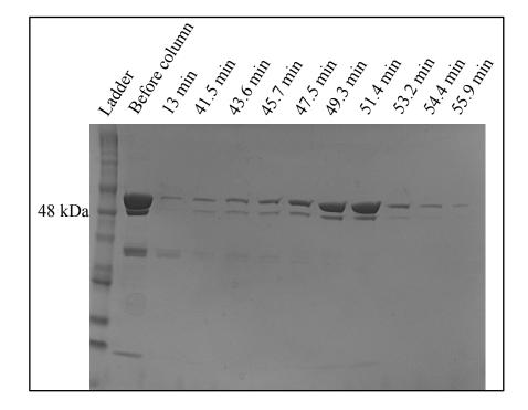
**Figure 12.** SDS-PAGE confirming mKATE2-eGFP fusion (53.25 kDa) purity after ion exchange chromatography. Lane 1: molecular weight ladder. Lane 2: mKATE2-eGFP fusion before ion exchange chromatography. Lanes 3-12: mKATE2-eGFP fusion elution from various minutes (min) throughout the gradient elution.
