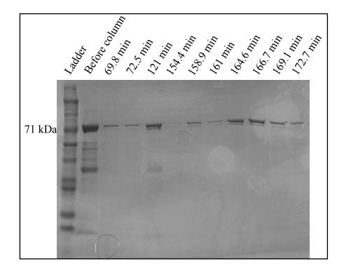
Figure 10. SDS-PAGE confirming HS1-monoHis (65 kDa) purity after ion exchange chromatography. Lane 1: molecular weight ladder. Lane 2: HS1 sample before ion exchange chromatography. Lanes 3-12: HS1 elution from various minutes (min) throughout the gradient elution.
