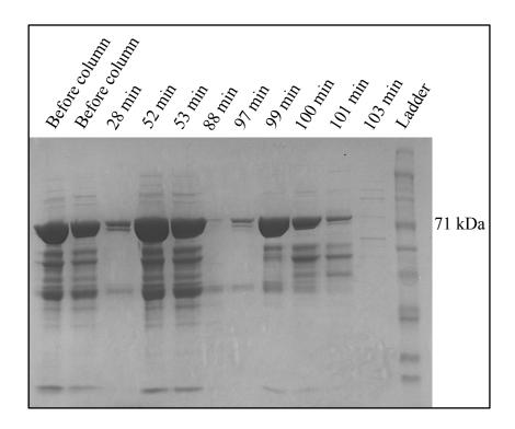
**Figure 7.** SDS-PAGE after TEV digest and Ni column to obtain HS1 (65 kDa) without the his<sub>6</sub>-tag. Lanes 1-2: HS1+TEV before running on Ni column. Lanes 3-11: HS1 elution from various minutes (min) throughout the low imidazole elution. Lane 12: molecular weight marker.
