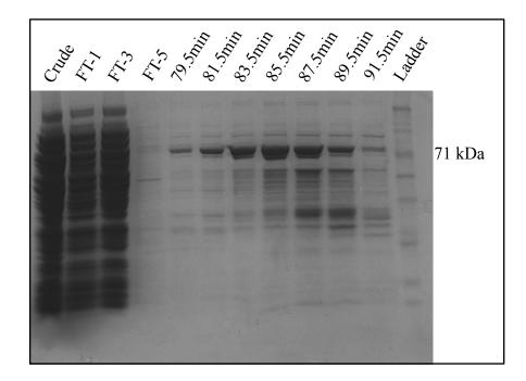
Figure 6. SDS-PAGE confirming efficiency of Ni column for HS1 (65 kDa) purification. Lane 1: HS1 crude lysate. Lanes 2-4: HS1 flow through in low imidazole wash. Lanes 5-11: HS1 elution from various minutes (min) throughout the gradient elution. Lane 12: molecular weight ladder.
