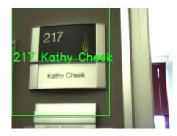
Figure 73: This sign is recognized and a measurement is made in the mapper. Google-Goggles has read both the room number and the text, so this sign can be used for data association.
