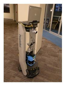
Figure 37: The robot platform used for these experiments. The camera attached to the laptop is the one that is used to detect the AR ToolKit Plus markers.
