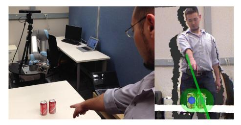
Figure 88: (Left) Our approach allows a robot to detect when there is ambiguity on the pointing gesture targets. (Right) The point cloud view from robot's perspective is shown. Both objects are identified as potential intended targets, therefore the robot decides that there is ambiguity.
