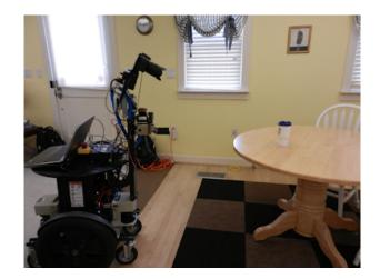
Figure 63: The robot platform used in this work. Point cloud data is collected with the Asus Xtion Pro camera, and laser scan data is collected with the Hokuyo UTM-30. Both of these sensors are placed on the gripper near the middle of the robot. The Asus camera is mounted upside-down on top of the gripper for more rigid and repeatable attachment.
