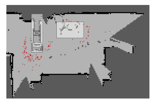
Figure 106: The area mapped by our system with relevant locations labeled, and person measurements shown in red.
