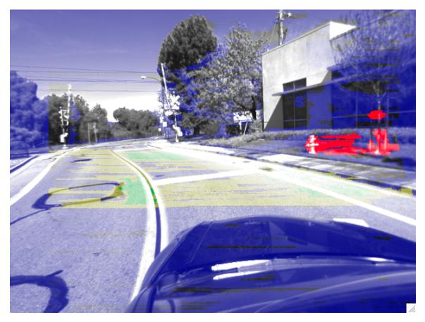
Figure 19: An example of the obstacle detection. Any connected component not part of the road is considered as an obstacle.
