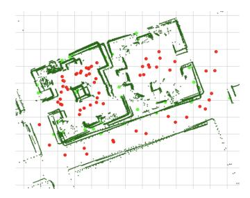
Figure 46: The initial state of the map, before optimization. Poses are shown in red, static landmarks are shown in green. The dark green points are laser scans, and are for visualization purposes only.
