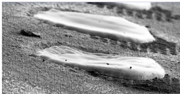
Figure 4.14 Surface of plated copper posts in the Syron carrier.
