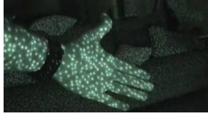
Figure 36: Kinect IR dot pattern used to estimate depth.
