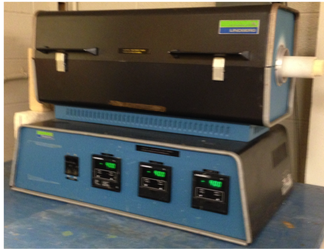
Figure 3.4: Lindbergh tube furnace used for isotropic coarsening.
