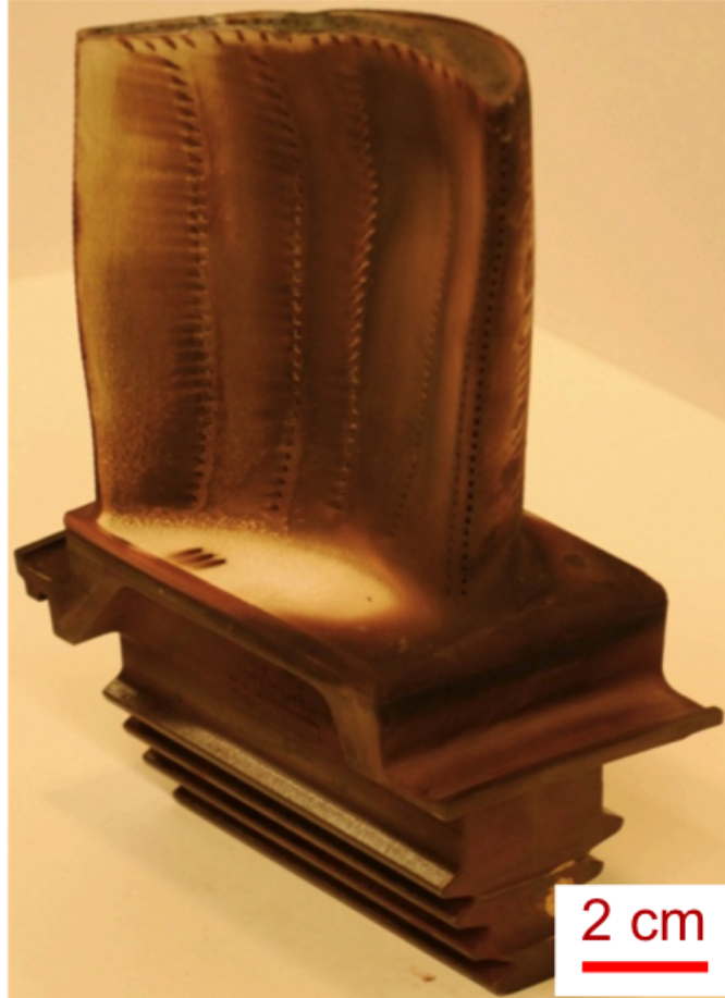
Figure 4.6: Second stage airfoil from a Siemens Energy SGT500 IGT removed from service after 32,000 hrs.
