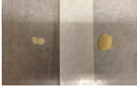
Figure 3.14 Pictures of Ag coated Ni particles before (left) and after iodination for 1 minute (right).
