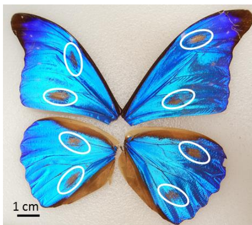
Figure 36. Error analysis of the peak reflection wavelength across an entire butterfly. Optical image of the four butterfly wings from a single butterfly. White circles denote the 8 separate areas from which scales were acquired. All 144 reflection spectra were acquired from single scales dispersed on a glass slide from one of the two butterflies. A \pm one standard deviation range from two separate butterflies was \pm 6 nm. This error was applied as the minimum error associated with measuring the peak wavelength from scales acquired from separate wing section areas.
