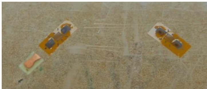
Figure 5-12 Image of the strain gages and lead wire terminal ready for strain gage positioning.
