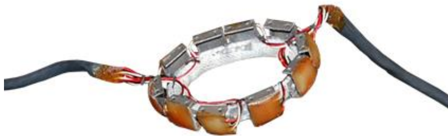
Figure 5-21 Photograph of a size 24 Physio™ ring instrumented with 10 suture force transducers.
