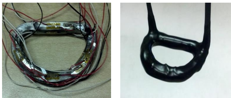
Figure 5-15 Left: Transducer's strain gages and lead wire terminals are coated in Loctite® M-31CLTM Hysol® Medical Device Epoxy (Step 8); Right: Following harnessing the transducer's wires (Step 12) , the entire transducer is dip-coated in synthetic rubber (Step 10).
