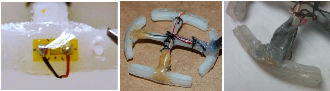
Figure 5-9 Left: Strain gage coated with epoxy (Step 9); Center: strain gages coated with nitrile rubber (Step 10); Right: application of 3145 silicone with the measurement arm cushions in place (Step 12).
