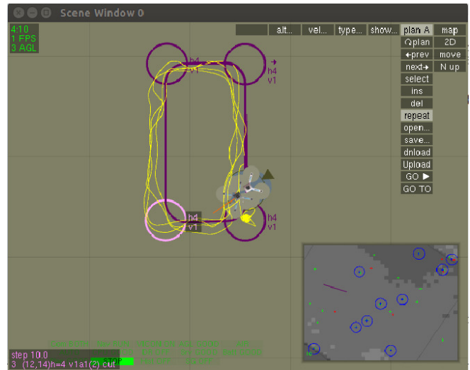
Fig. 7. GUST Quadrotor running Vision navigation simulation of track similar to vicon room. Two quadrotor vehicles can be seen. One is actual the other is where the navigation system thinks it is.
